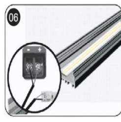
6. Connect the power & IP65 attention
